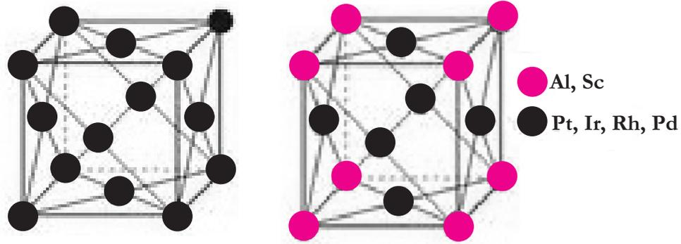
**Figure 1:** Crystal Structure for Pure Iridium, Platinum, Rhodium and Palladium (left). Crystal Structure in which one Atom of Iridium, Platinum, Rhodium and Palladium have been replaced with either Aluminum or Scandium (right). This latter structure type is designated as  $L1_2$  in the Strukturbericht notation or as  $cP4$  in the Pearson's symbol (space group  $Pm-3m$ ).
