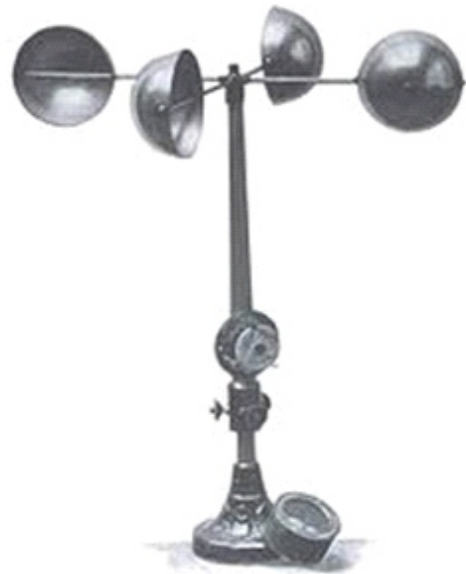
Figure 9: Cup Anemometer (Encyclopaedia Britannica, 2012)
